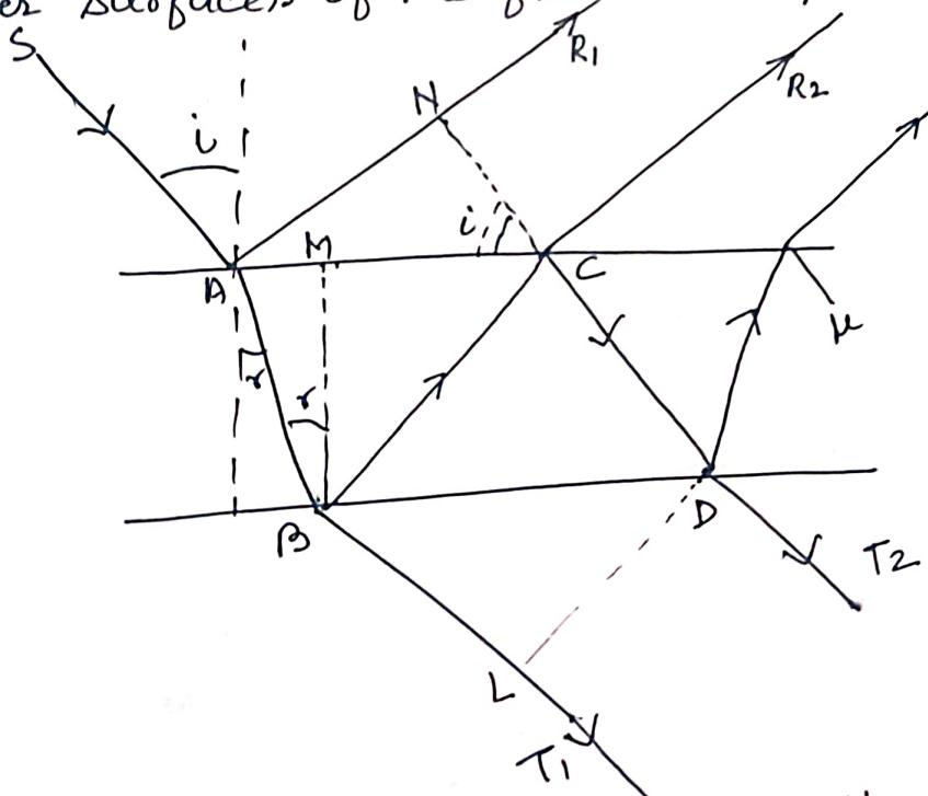
Interference of light by parallel sides thin film
